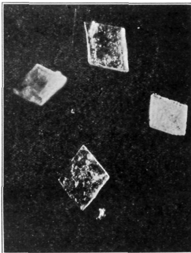
Fig. 1.—Crystals of monomeric ethylene oxalate. \times 94 . (These crystals were placed for observation in a microscopic culture plate and sealed against the access of air and moisture by means of a cover glass. Mechanical disturbances were avoided, and subsequent observations, except the last, were made from exactly the same position as the first.)
